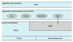
Below is kernel consisting of Mach microkernel and BSD Unix parts, plus I/O kit and dynamically loadable modules (called kernel extensions)
